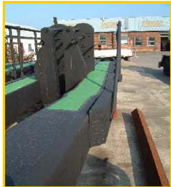
Epoxy base/grit surface
